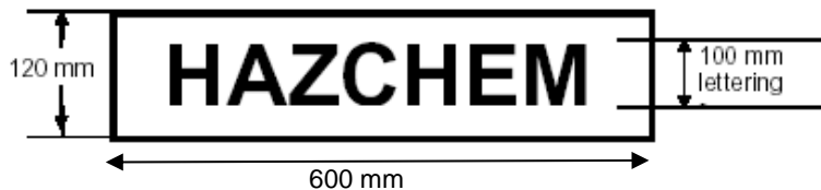
Figure 13.1 Form and dimensions of outer warning placard
